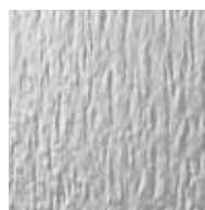
E1 Embossed 1 16 Gauge Stainless Steel
